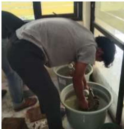
proses perendaman benda uji CBR soaked
