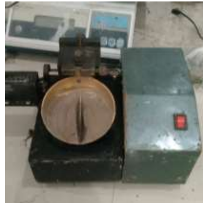
Proses penentuan batas cair
