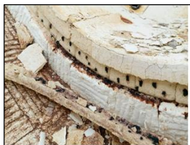
Gambar 4. Serpihan Material Castable Refractory
