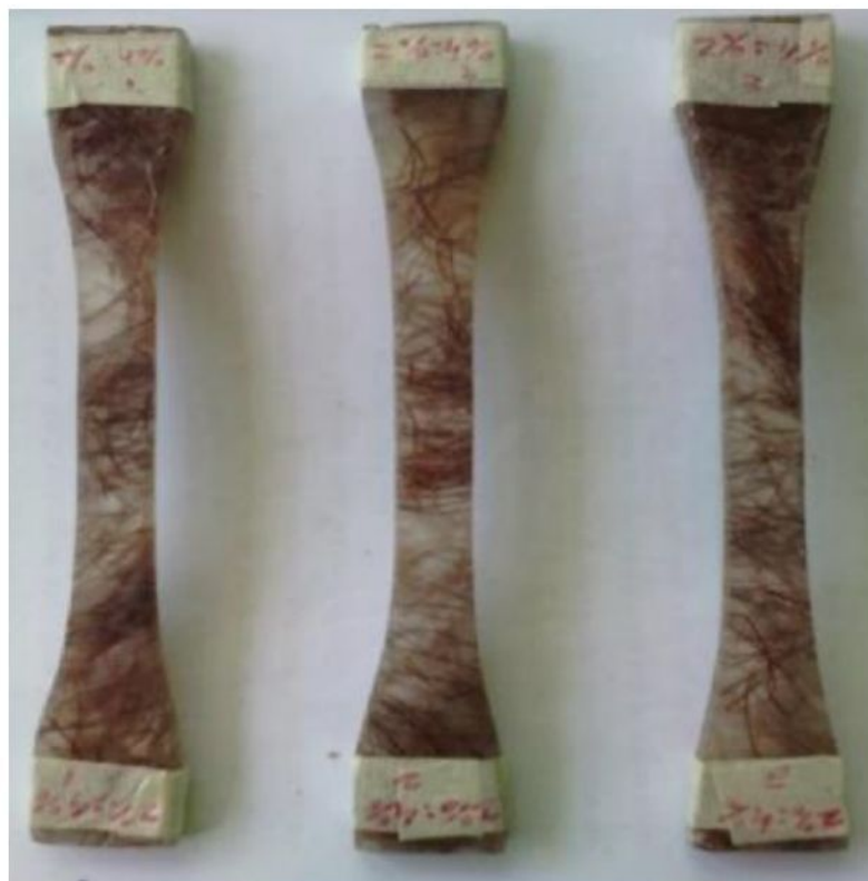
Gambar 4. 6 69% resin, 2% fiber glass dan 4% serat gambas
