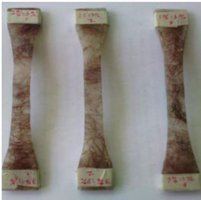
Gambar 4. 4 94% resin, 3% fiber glass dan 3% serat gambas
