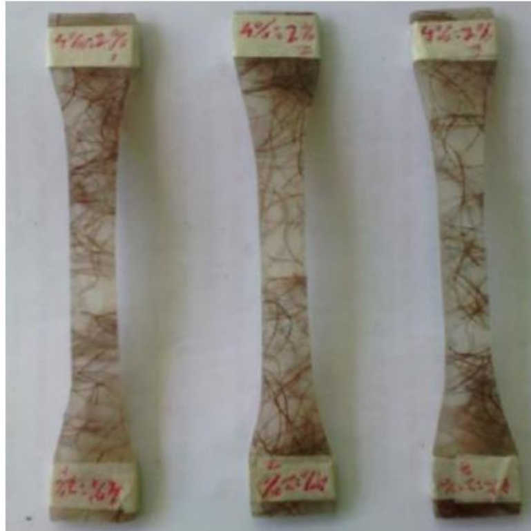
Gambar 4. 5 94% resin, 4% fiber glass, dan 2% serat gambas
