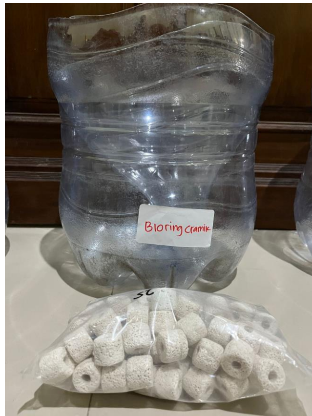
Gambar 8. Filter Bioring Cramic
