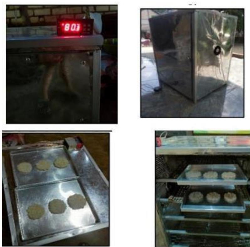
Gambar 5. 1 Implementasi dari alat Microcontroller Based Food Dehydrator for Rengginang Crackers
