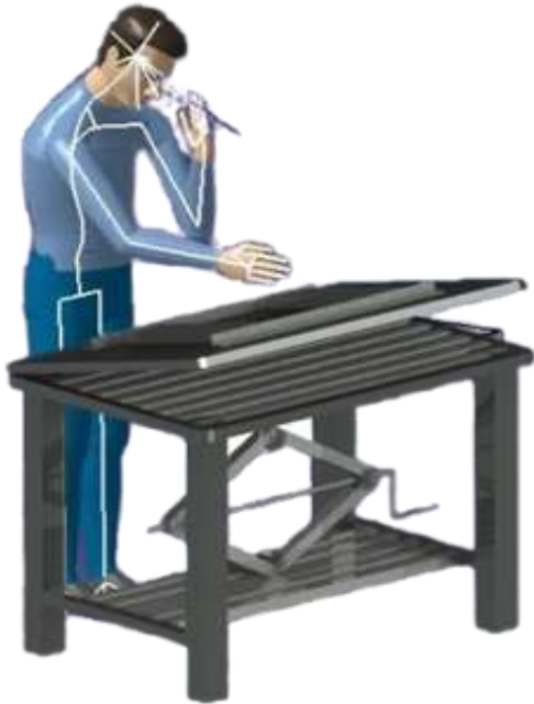
Fig. 4 Virtual Environment Of Human Model Simulation Testing With A Validated Welding Workbench Design Concept.
