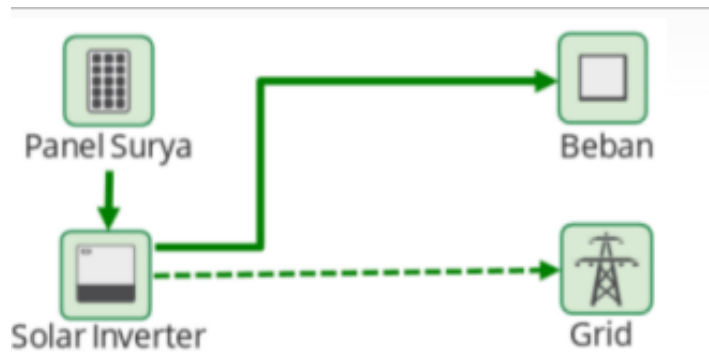
Gambar 2. 3 Skema system on-grid
