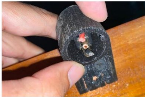
Gambar 4. 4 Pemasangan Housing Switch
