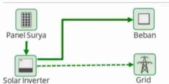
Gambar 2. 3 Skema system on-grid
